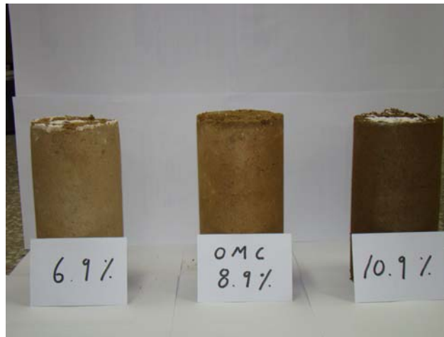
Fig. 3 Prepared test samples at different water contents
