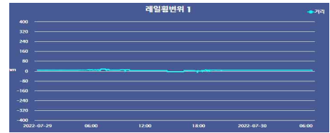
(c) Measurement result on rail displacement
