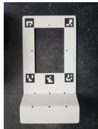
Fig. 1 Measuring ruler using Aruco marker
