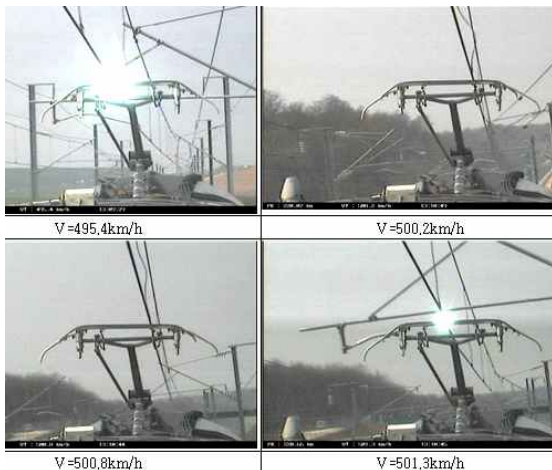
Fig. 1 The current collection images near 500km/h when 575km/h test in France.
