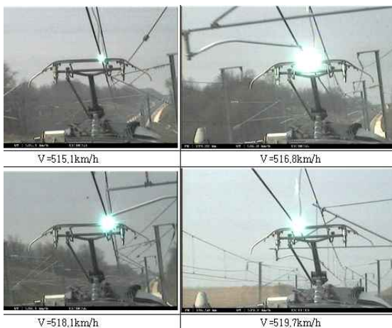
Fig. 2 The current collection images in passing 500km/h when 575km/h test in France.
