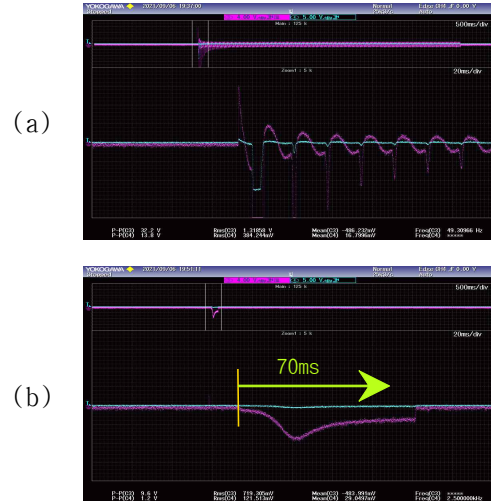
Fig. 5 Exp. results (a) AC with no trip of MCB, (b) DC with trip of MCB.
