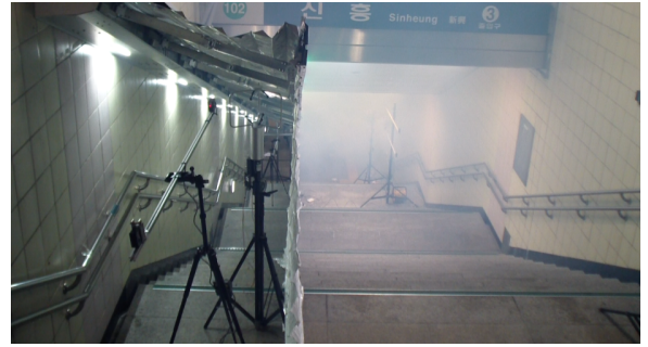
Fig. 3 Scene of smoke blocking for evacuation passage
