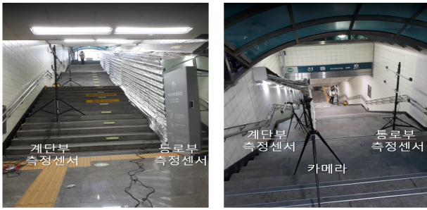
Fig. 2 Smoke barrier test for deployable evacuation passage
