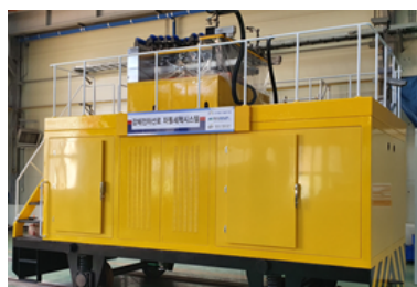
Fig. 3 Automatic cleaning system for ROCS (Rigid Overhead Conductor System)
