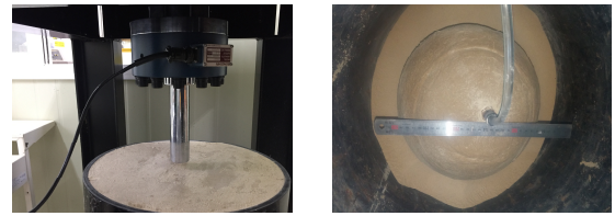
(a) Measurement of Stiffness (b) Confirmation of Injection Fig. 4 Miniature Cyclic Plate Loading Test
