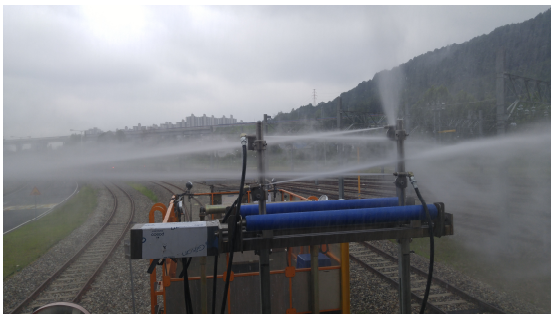
Fig. 1 Test-made injection nozzle
