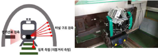
Fig. 2 Method of detection Tunnel-Imaging device)
