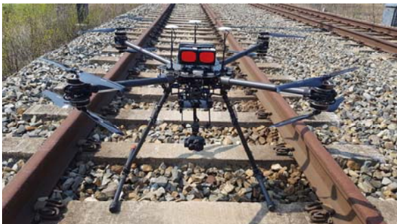
Fig 1 Drone for Inspection Crack on Track
