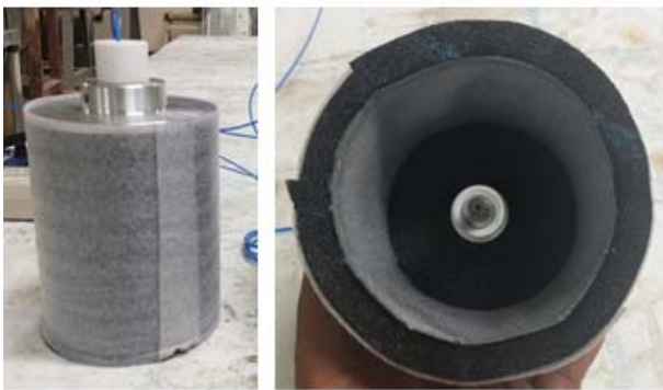
Fig. 2 A prototype of an air-coupled sensor in IE testing.
