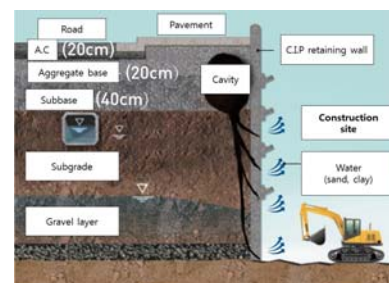
(b) Inflow of excavation construction site
