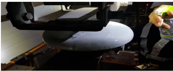
Fig. 1 Pollution cleaning test using spray
