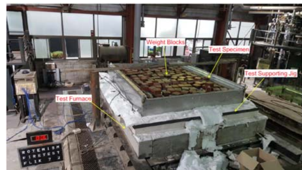
Fig. 3 Setup Test Specimen
