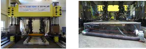
Fig. 1 Static loading test to determine the optimum thickness and analyze characteristics of curved part of AC track-bed
