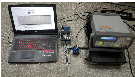
Fig. 1 System for checking collected data: waveform generator, linear power amplifier, vibrator, geophone, Ni DAQ, alternative DAQ and notebook
