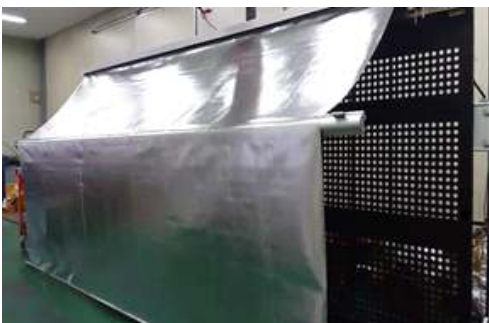
Fig. 2 On wall type deployable safe pathway
