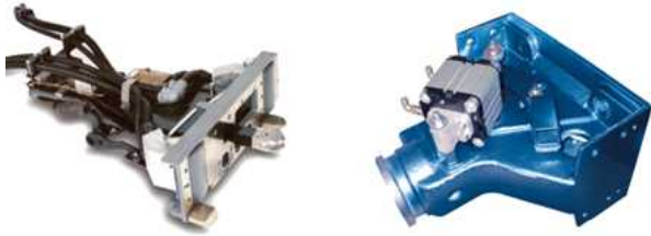
Fig. 6 Wedge-lock / Tomlinson Coupler
