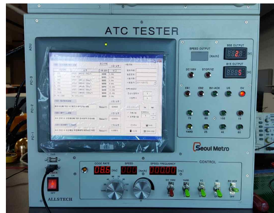
Fig. 7 Developed ATC Test Equipment (Fixed Type)
