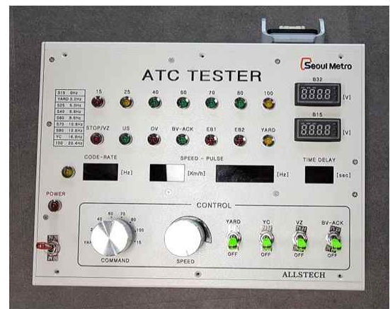
Fig. 8 Developed ATC Test Equipment (Portable Type)
