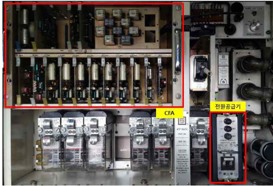
Fig. 4 CFA and Power Supply for ATC Onboard Signal Equipment
