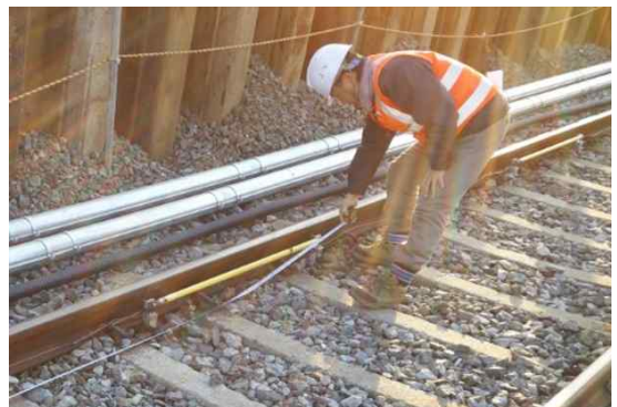
Fig. 1 On-site rail mounted measurement sensor
