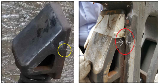
Fig. 3 Locked between friction block and side-frame
