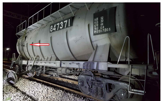
Fig. 1 Derailed accident freight vehicle
