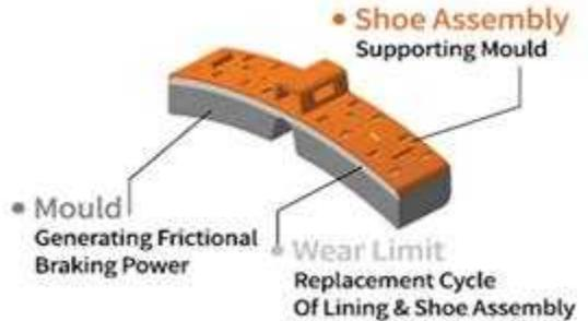
Fig. 3 Brake Shoe for Tread Brake
