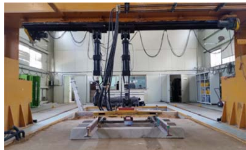
Fig. 3 View of static and cyclic loading test
