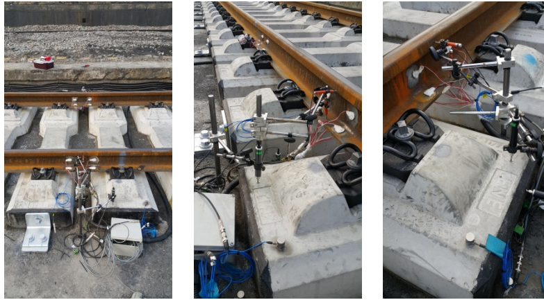
Fig. 3 Arrangement of L.V.D.T.s and strain gauges in wide sleeper type asphalt concrete track
