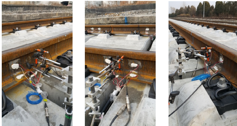
Fig. 3 Arrangement of L.V.D.T.s and strain gauges in panel-type asphalt concrete track
