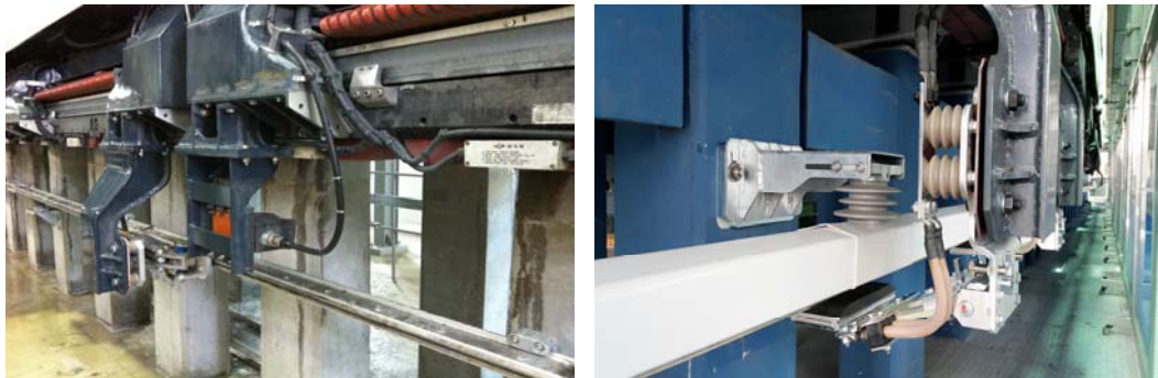
Fig. 2 Type of the Third-Rail feeding Method of Maglev
