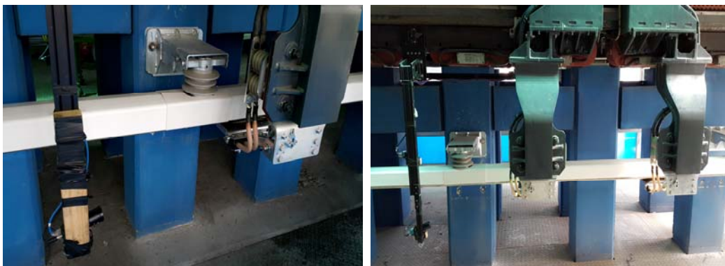
Fig. 4 Test Equipment of the Maglev Current Collector Device
