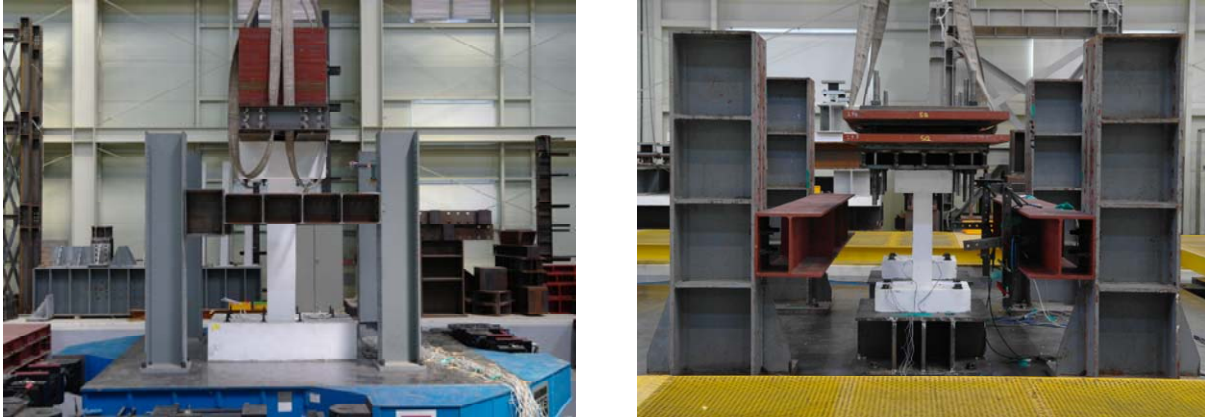
Fig. 1 Test setups for prototype (left) and model (right)
