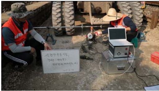
Fig. 3 Plate loading test
