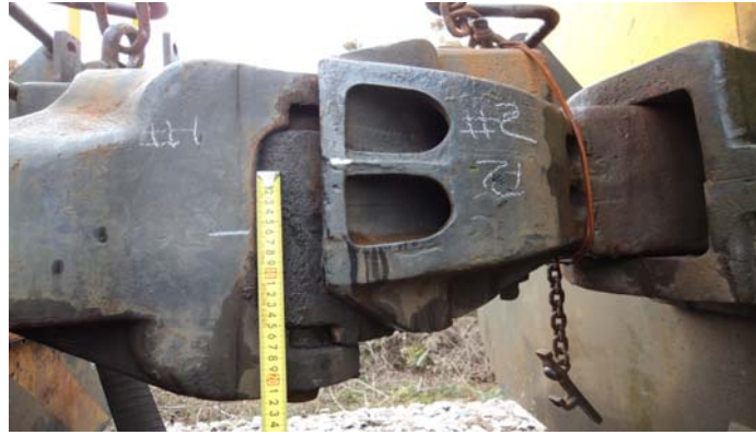
Fig 2. Difference height of the coupler between rolling stock
