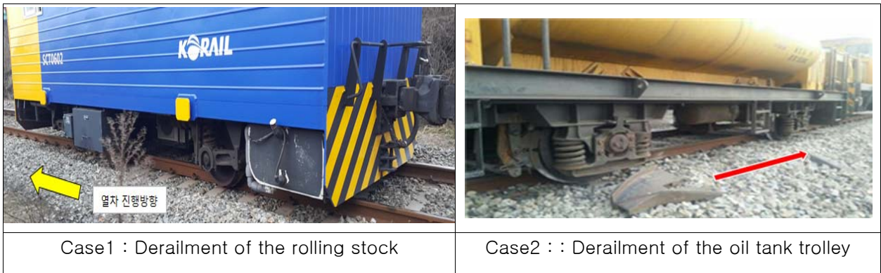
Fig 1. Derailment of the maintenance equipment
