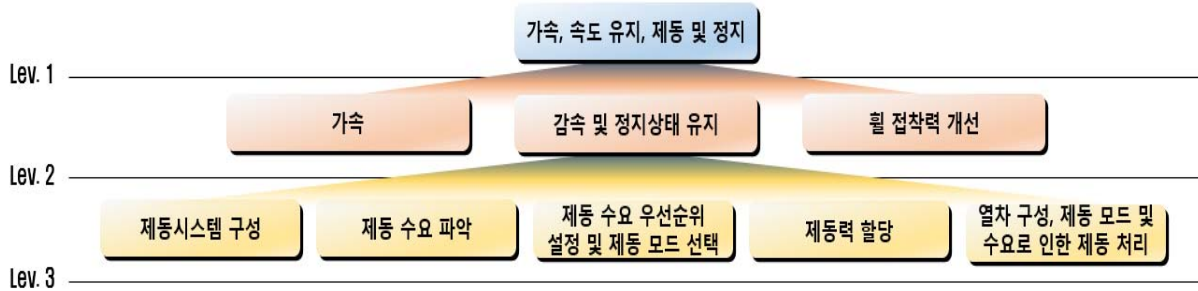
Fig. 2 Level 3 FBS for Brake system
