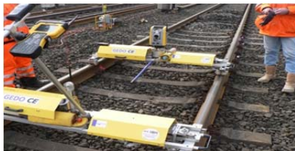
Fig. 1 Typical measuring equipment of track linearity (GEDO)
