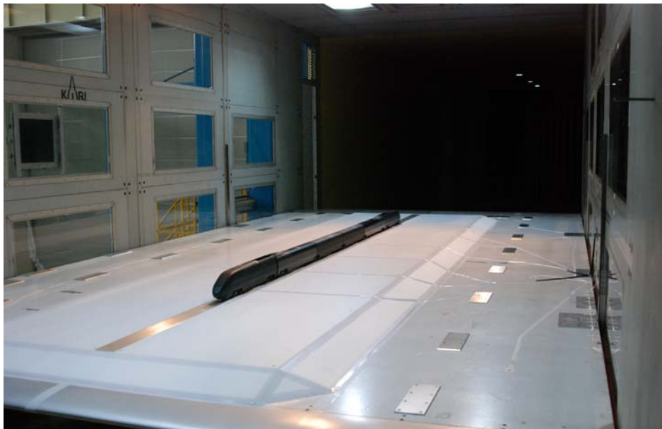
Fig. 3 Wind tunnel test model in the test section
