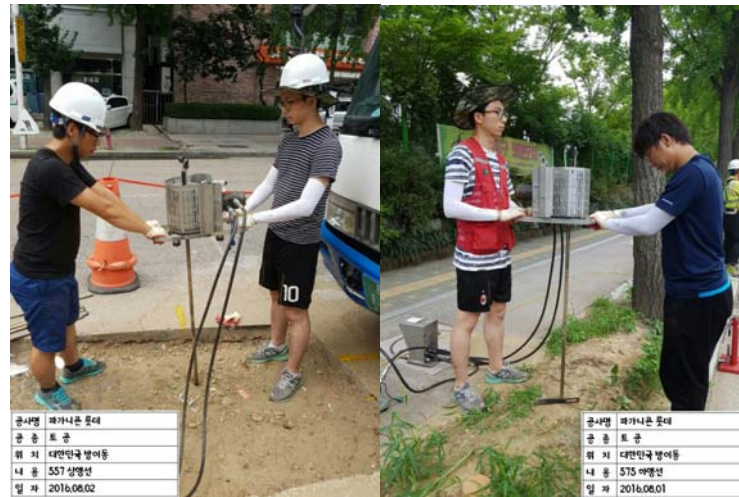
Fig. 4 Pagani cone test on the ground above the tunnel
