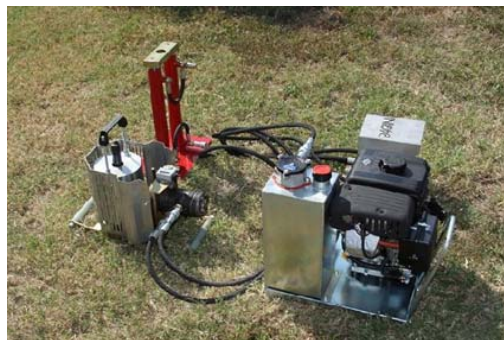
Fig. 3 Components of Pagani cone
