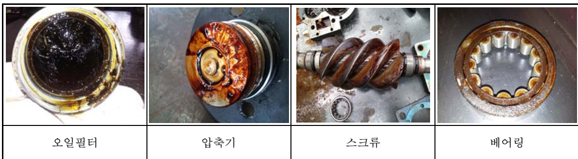
Fig.3 Associated fallouts caused by the oil discoloration
