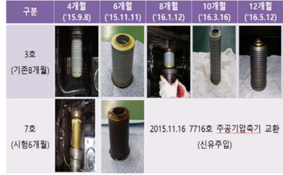
Fig.6 716 Train oil filter test results
