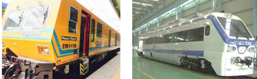
Fig. 2 Track inspection Train (EM-140K, Roger-1000K)
