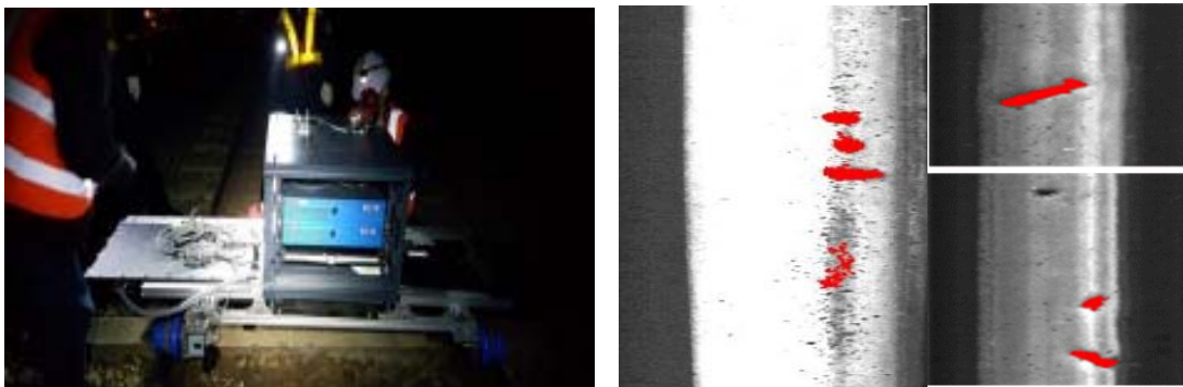
Fig. 5 Rail wear & Track defect inspection-equipment (Test)
