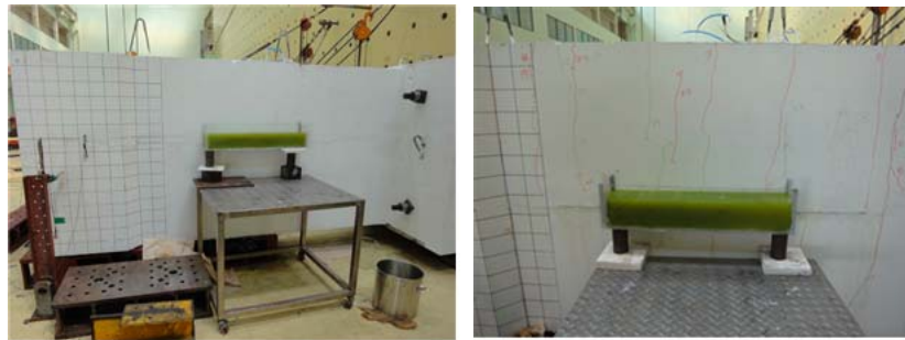
Fig. 3 Leakage Test during Structural Performance Experiment
