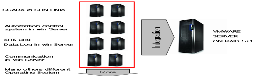
Fig. 6 The integrated various system to VMWARE on one server
