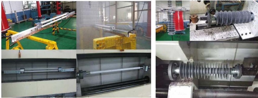
Fig.7 Performance test of Stem Insulator and Section Insulator for Overhead Rigid Conductor Rail
