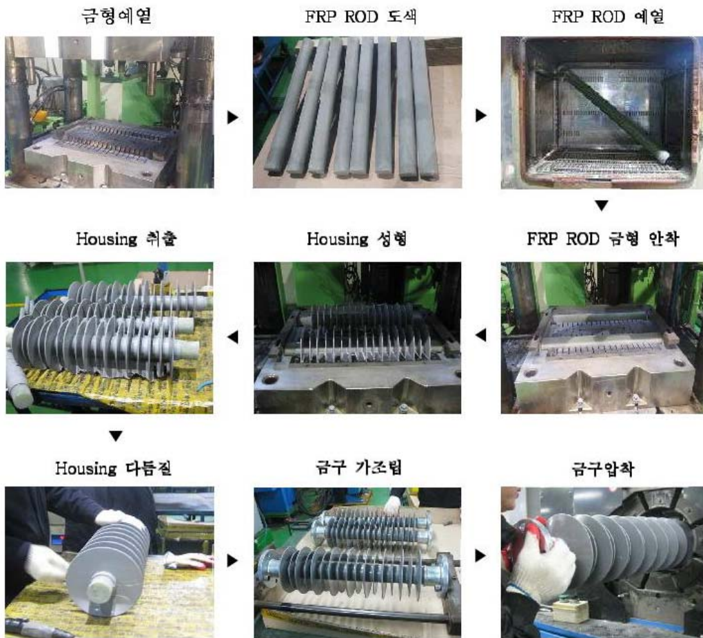
Fig. 5 Production process of Stem Insulator for Overhead Rigid Conductor Rail
