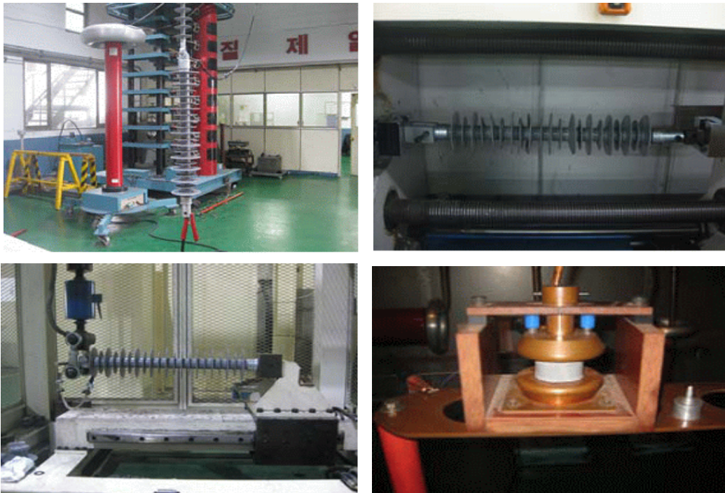
Fig6. Performance test for Polymer Insulator for Contaminated Area
