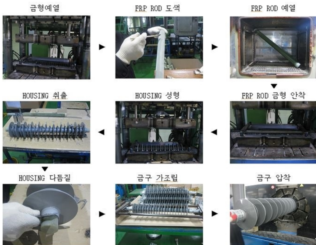
Fig. 4 Production process for Polymer Insulator for Contaminated Area
