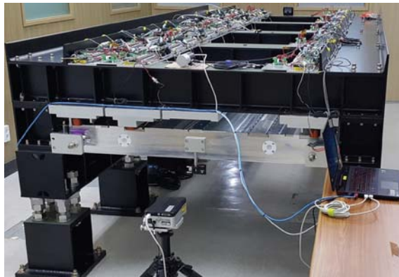
Fig. 1 The High accuracy magnetic levitation transport system
