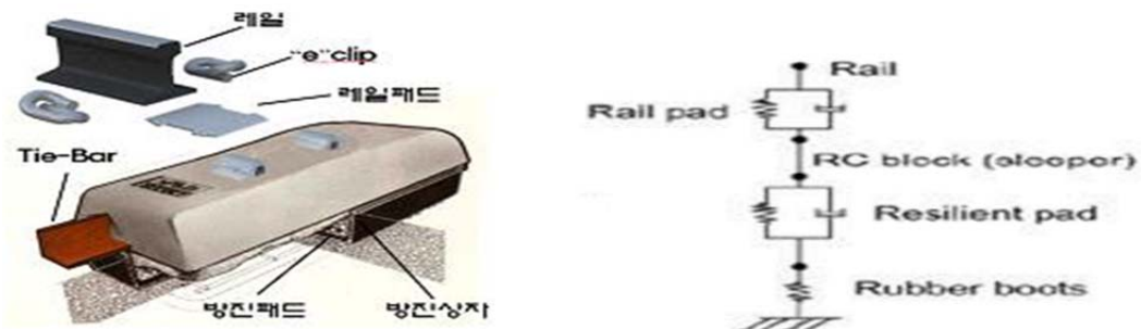
Fig. 2 STEDET Track Component materials and Spring Model
