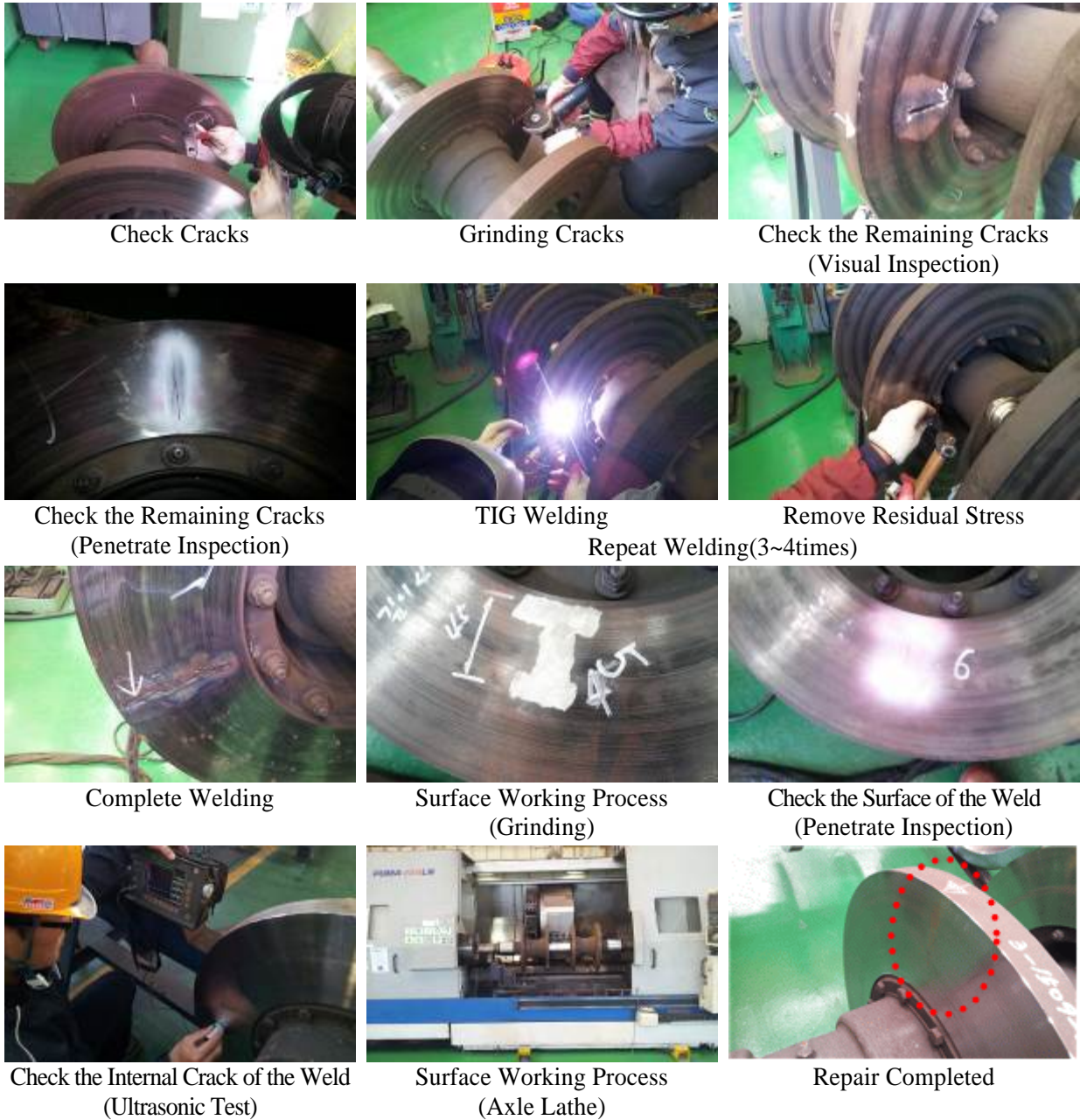
Fig. 4 Brake Disc Repair Procedure Weld
