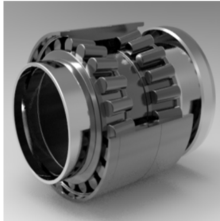
Fig. 1 The 3D modeling of the axle bearing (DRTRB)
