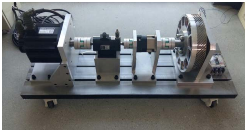
fig. 2 Entire system of eddy-current brake
