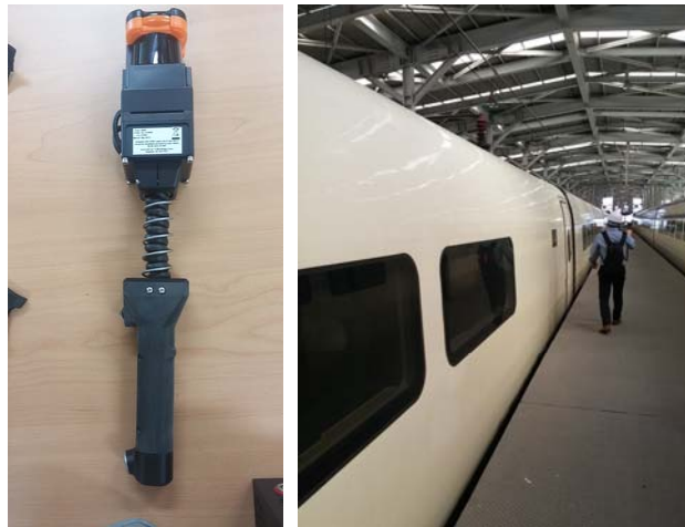
Fig. 2 The used handheld mobile mapping system and relative position measurements of train positioning sensors installed on HEMU-430x
