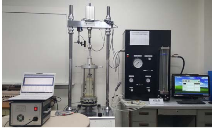
Fig. 1 Cyclic triaxial compression test
