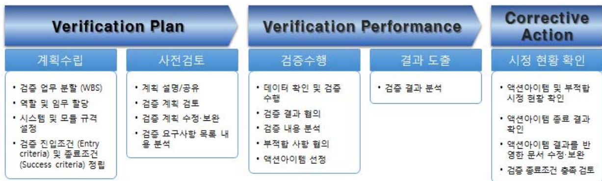
Fig. 4 Verification process for the automatic coupler
