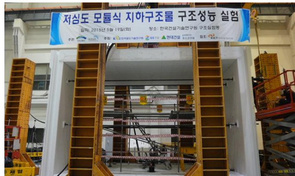
(b) Full-scale of box structure
