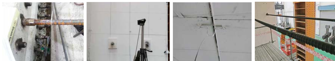
(a) Strain gauge (Steel) (b) Displacement gauge (c) Crack gauge (d) Strain gauge (Steel rods)
